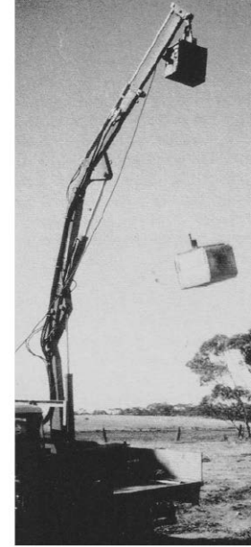
Figure 11.4 Impact source. A half-ton weight being dropped from a portable crane during a survey of the low-velocity layer.
