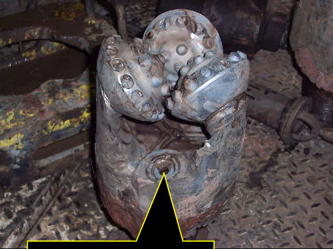
Openings (nozzles): Entry point for borehole mud
