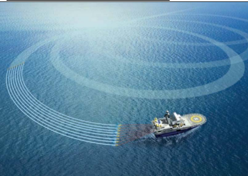
FIG. 2.40 Typical acquisition patterns for conventional 3D surveys. (A) Racetrack and (B) antiparallel survey patterns.
